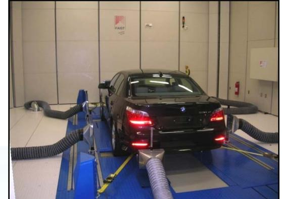
4-Wheel Chassis Dynamometer
