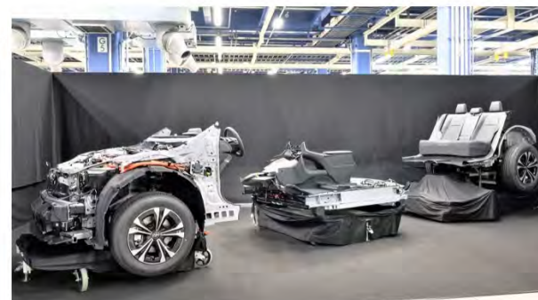
Toyota's next-generation electric vehicles will be produced in three modular sections. (Photo courtesy of Toyota)
