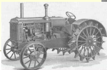
1935-1940 Brochure Photo of an IHC, McCormick Deering WD-40 (Diesel) tractor equipped with steel wheels. This was the first Diesel powered wheel tractor built in the United States.
