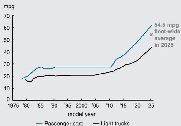
NOTES: The figure displays the evolution of corporate average fuel economy (CAFE) standards—measured in miles per gallon (mpg)—for new passenger cars and light trucks in the U.S. See the text for further details.
