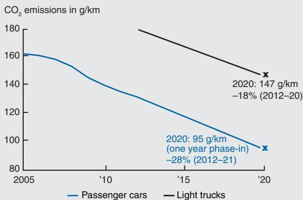
NOTES: The figure displays the evolution of carbon dioxide (CO<sub>2</sub>) emissions standards in grams per kilometer (g/km) for new passenger cars and light trucks in the European Union. The CO<sub>2</sub> emissions rate is a measure of fuel economy. See the text for further details.
