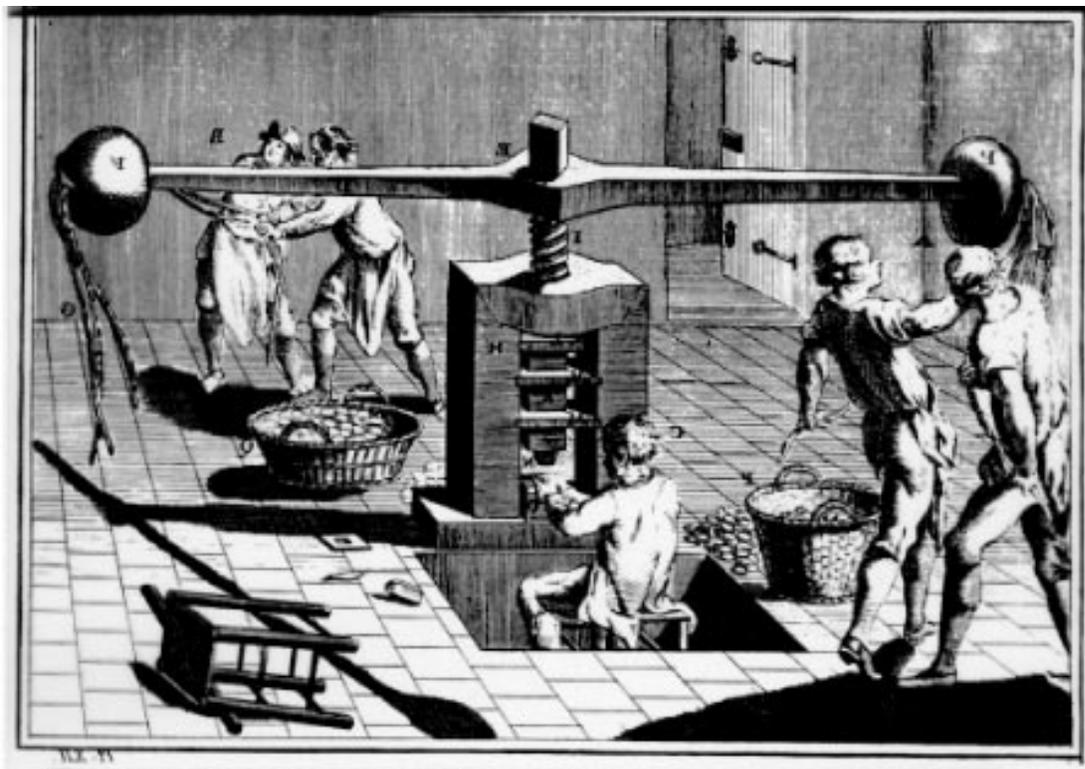
**Figure 2:** The screw-press (engraving for Diderot's *Encyclopédie*, ca. 1755).
