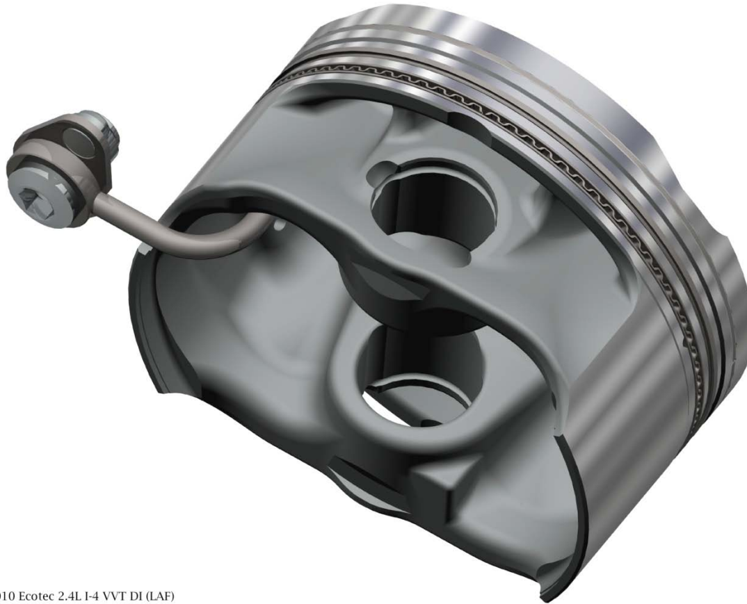
2010 Ecotec 2.4L I-4 VVT DI (LAF) Piston Head and Oil Cooling Jet
